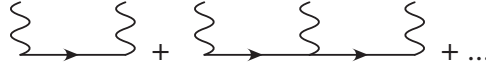
Figure A.1. The diagrams taken into account when calculating the self-energy for the trapped polaron in the high temperature limit.
